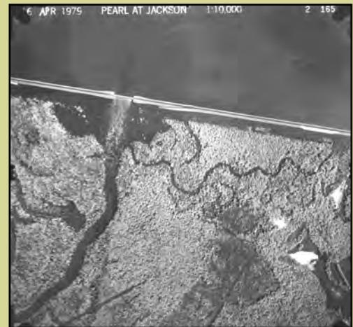
This satellite image from the Easter flood of 1979 shows The Rez at its highest recorded level - 299.79 - and highest release rate - 140,000 cubic feet per second. That's water on both sides of the dam.
